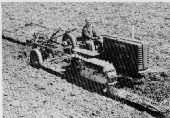
Tough and tireless, the Model "MC" provides dependable, economical power for all seedbed preparing jobs. Here it is shown with three 14-inch bottoms plowing 7 inches deep.
